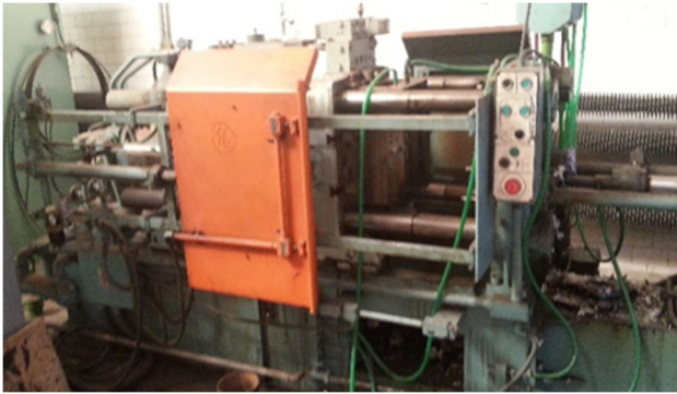
Fig. 2 Pressure die casting machine CLOO 100/16-B2
