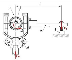
Fig. 1 The measuring principle 1 - measuring head, 2 - shaft, 3 - sliding bearing, 4 - arm, 5 - force sensor, 6 - transmission mechanism
