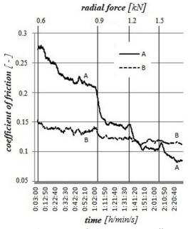
Fig. 4 The course of the average coefficient of friction in the bearings A and B
