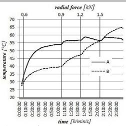
Fig. 3 The course of average temperature in the particular bearing A and B
