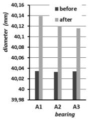
Fig. 5 The average values of the diameter of the bearings A before and after the experiment
