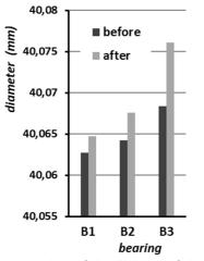
Fig. 6 The average values of the diameter of the bearings A before and after the experiment
