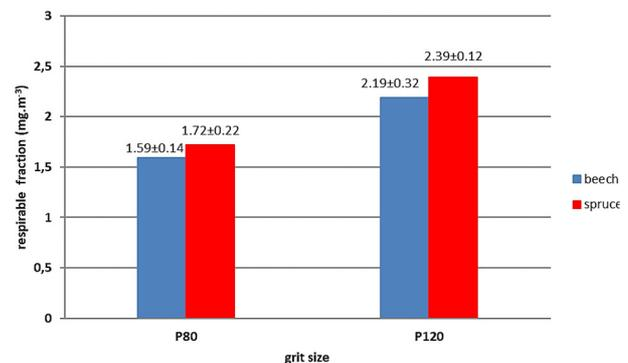
Fig. 3 Effect of wood species and abrasive grain size on respirable fraction of wood dust mass concentration
