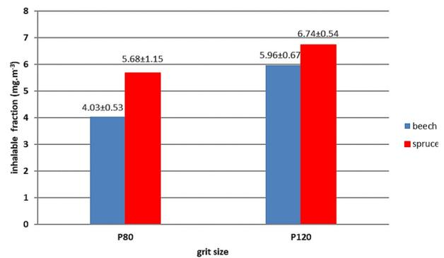
Fig. 2 Effect of wood species and abrasive grain size on inhalable fraction of wood dust mass concentration
