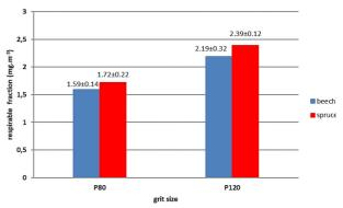
Fig. 3 Effect of wood species and abrasive grain size on respirable fraction of wood dust mass concentration
