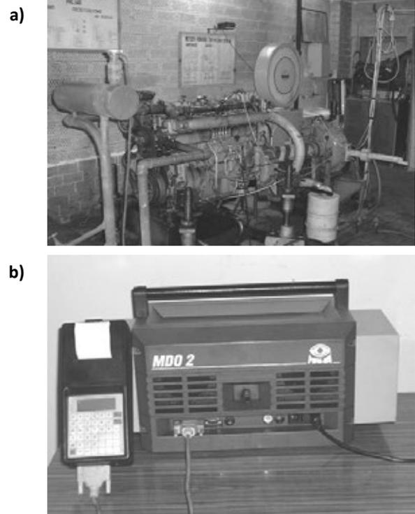
**Fig. 2** Test bench with an engine of 359 type (a) and MAHA MDO-2 opacimeter (b)
