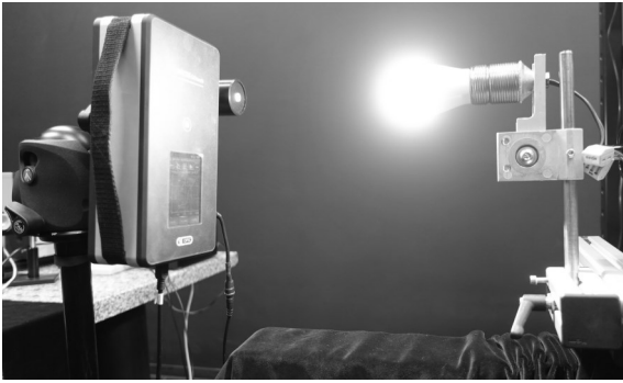
Fig. 5 View of the measuring set for the spectral distribution of a light source
