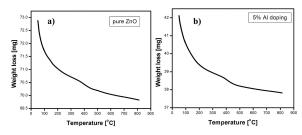
Fig. 9. (a) TGA curve of pure ZnO nanoparticles and (b) TGA curve of of 5 % Al doping ZnO nanoparticles
