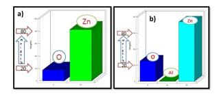
Fig. 3. (a) weight % versus composition of pure ZnO sample and (b) weight % vs. composition of 3 % Al doped ZnO sample.
