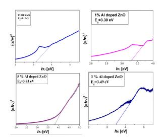
Fig. 6. Tauc plots to estimate band gap of pure ZnO and Fig. 7. Energy band gap variation with aluminum Al Al doped ZnO NPs.
