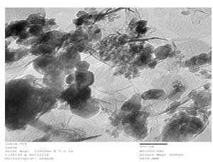
Fig. 4. TEM image of 1% Al doped ZnO nanoparticles calcined at 500 °C.
