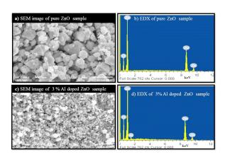
Fig. 2. SEM and EDX images of pure and 3 % Al doped ZnO nanoparticles.
