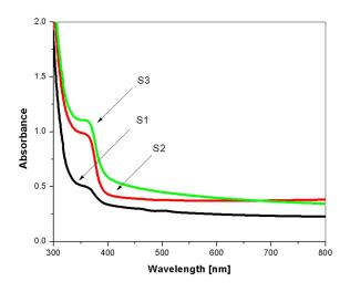
Fig. 5. UV-Vis absorption spectra of ZnO thin-films.
