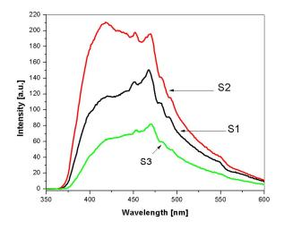
Fig. 4. Photoluminescence spectra of ZnO-thin-films on glass substrates.
