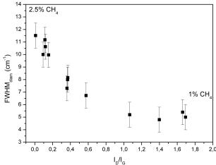
Fig. 7. The correlation between FWHM $_{dia}$  and  $I_D/I_G$  ratio.
