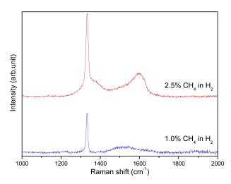
Fig. 3. Typical Raman spectra of two diamond films synthesized at different deposition conditions: with different CH<sub>4</sub> working gas concentrations.
