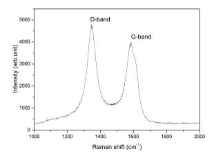
Fig. 1. Raman spectrum of amorphous carbon.
