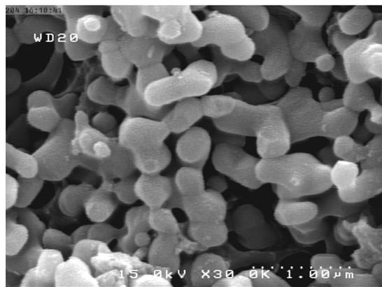
Fig. 2. SEM image of the surface of an  $\alpha$ -Al<sub>2</sub>O<sub>3</sub> support.
