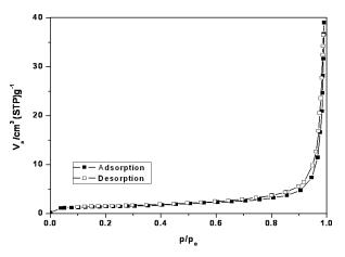
Fig. 5. Nitrogen adsorption-desorption isotherm of a SrO sample synthesized using chemical combustion at 1000 °C for 5 min.
