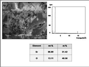
Fig. 4. SEM image and EDS analysis of a SrO sample prepared by chemical combustion at 1000 °C for 5 min.
