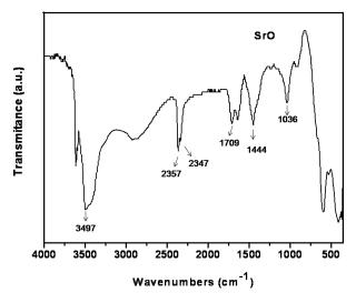
Fig. 3. IR spectrum of SrO synthesized by chemical combustion at 1000 °C for 5 min.
