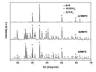
Fig. 1. XRD patterns for the SrO powders prepared using combustion method at a molar ratio of strontium nitrate to urea 1:1, at different temperatures, for 5 min.
