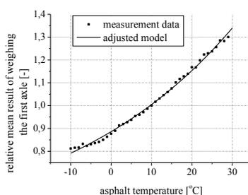
Fig. 5. Temperature characteristics of a WIM system within the range of  $-10$  to  $30^\circ\text{C}$  ( $14 - 86^\circ\text{F}$ ).
