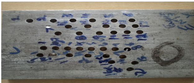
Figure 1: Drilled stainless steel plate.
