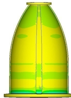
Fig. 20 - OW + PS + HP– Vertical stresses \sigma_z – outside and inside surface (daN/cm 2 )
