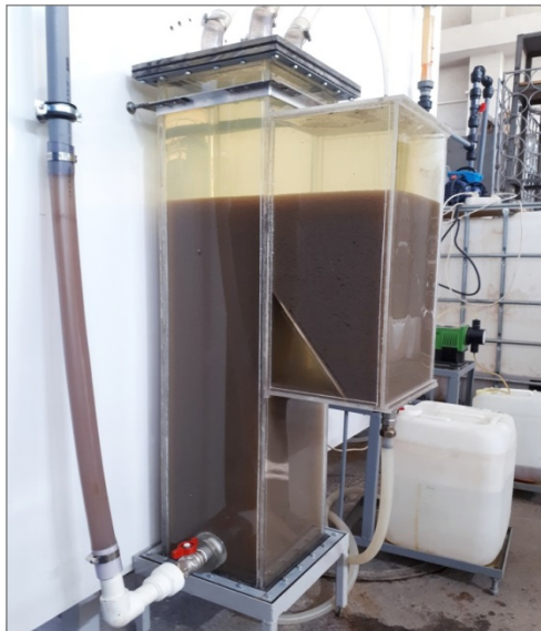
Fig.10. Sludge settled at the bottom surface of the inlet, and sludge collector chambers.
