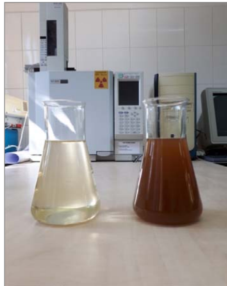
Fig.12. Samples of meat processing wastewater before and after chemical treatment.
