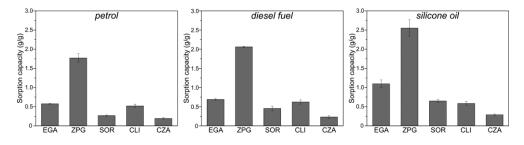
Fig. 4. Sorption capacities of materials used for the sorption of gasoline, diesel and silicone oil.
