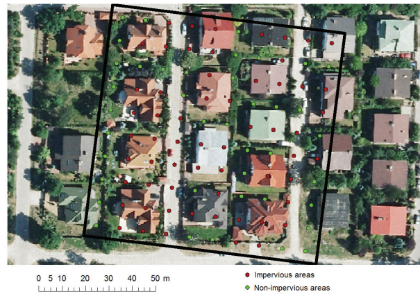
Figure 2. Example of sample with points regularly distributed every 10 m.
