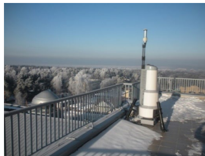
Fig. 6. Optical remote sensing complex ZephIR for measuring wind speed and direction at a distance up to height of 160 m on five height levels (located in Ventspils, site 3).
