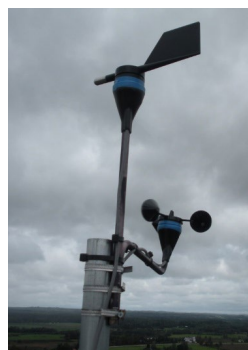
Fig. 2. Sensors for wind speed NRG #40, vane NRG #200, which are mounted on mast.
