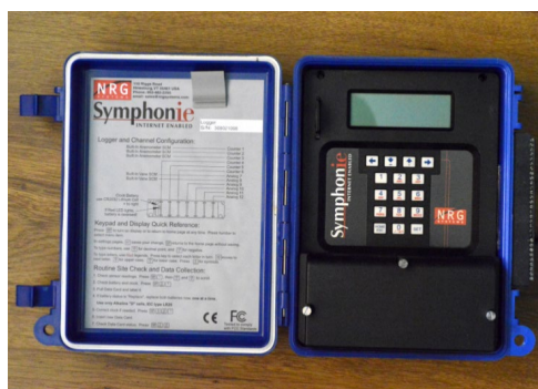
Fig. 1. Registration unit LOGGER Symphonie 9200 for recording data from sensors of wind speed NRG #40, vane NRG #200, temperature NRG #110s and air pressure NRG BR-20.
