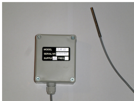
Fig. 4. First generation PT1000 wireless temperature measurement unit.
