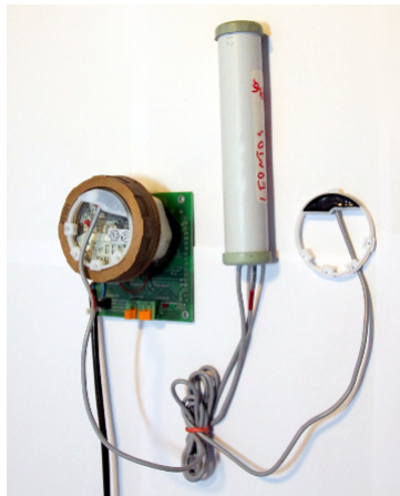
Fig. 3. Wireless impulse counter kit for water meter reading.
