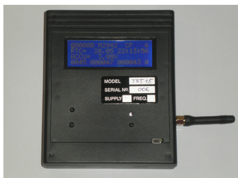
Fig. 2. Wireless data concentrator with non-volatile memory.
