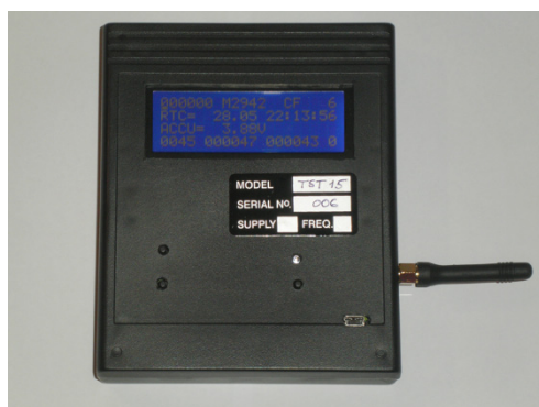
Fig. 2. Wireless data concentrator with non-volatile memory.
