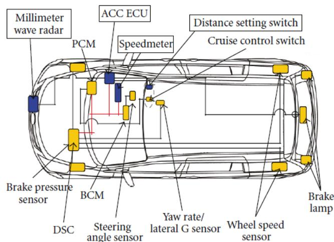
*Fig.2 ACC Vehicle Unit Components [Miyata S., et al 2010]*
