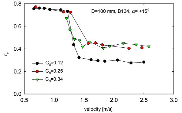
Fig. 5. Effect of the flow velocity  $V$  and slurry transport volumetric concentration  $C_d$  on chord averaged local concentration  $c_v$  in height  $y = 10$  mm above pipe bottom.
