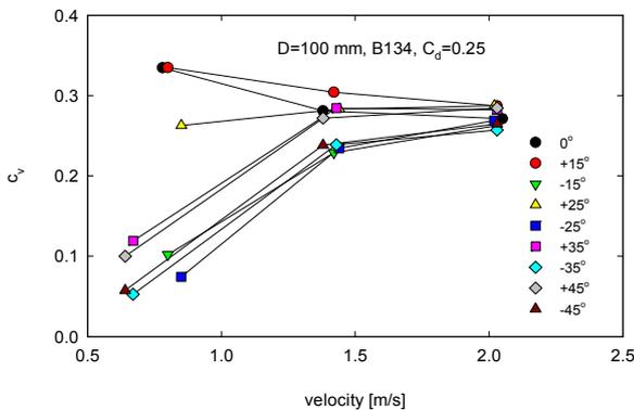
**Fig. 3.** Effect of the flow velocity  $V$  and inclination angle  $\alpha$  on the slurry in situ volumetric concentration  $C_v$  ( $C_d = 0.25$ )
