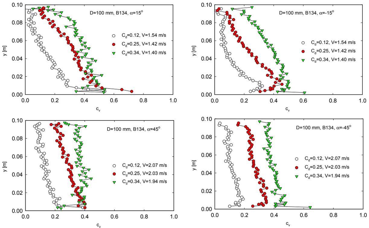
**Fig. 10.** Effect of transport concentration  $C_d$  on chord-averaged local concentration profiles for constant slurry velocity  $V$  and pipe inclination  $\alpha$ .
