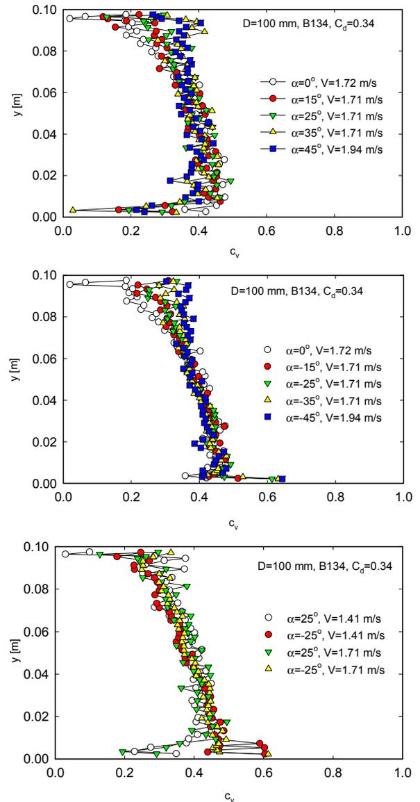
**Fig. 8.** Effect of the pipe inclination  $\alpha$  on chord-averaged local concentration profiles ( $C_d = 0.34$ ).
