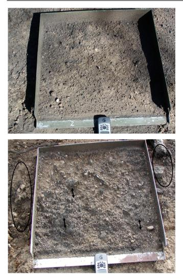
**Fig. 4.** Example plots from a) the burned 20% site, and b) the burned 60% site. The metal plot frames delineate the  $0.5 \text{ m}^2$  plot area from which the runoff and sediment samples were taken. Black ovals on b) show the rocks and stumps on site which can indicate macropores and increased ponding, while arrows highlight the rougher soil surface texture which slows surface flow and may increase infiltration.
