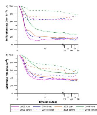
**Fig. 2.** Infiltration rate versus time for the rainfall simulator experiments on burned and control sites on a) 20% slope plots and b) 60% slope plots, in the year of the fire (2003), post-fire year 1 (2004), post-fire year 2 (2005), and post-fire year 5 (2008).
