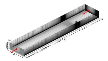
Fig. 2. Computational mesh for simulation with W = 7.3L. The arrow shows the flow direction.
