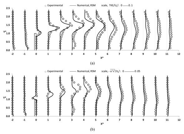
Fig. 7. Comparison of turbulence statistics between measurement and RSM model. a) Turbulent Kinetic Energy and b) Horizontal Reynolds stresses.
