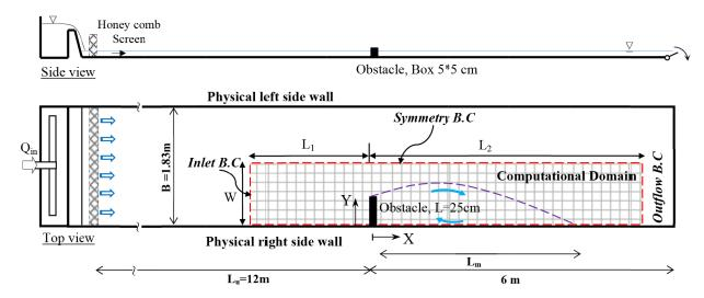
Fig. 1. Schematic representation of the experimental test case. The area denoted by red dashed lines shows the computational domain in the present numerical simulation.
