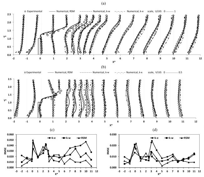
**Fig. 6.** Comparison between numerical and experimental results. a) Streamwise velocity component, b) Spanwise velocity component, c) Root Mean Square, RMS, between the numerical and experimental streamwise velocity component, d) Root Mean Square (RMS) between the numerical and experimental spanwise velocity component.
