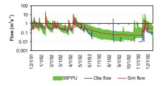
**Fig. 4.** Comparison of the hydrograph and uncertainty prediction at gauge 1. Obs flow represents measured discharge in impacted conditions and Sim flow represents the calibrated simulation in natural conditions. The shaded (green) interval is the 95% uncertainty predictions (P-factor = 0.41; and R-factor = 0.20).
