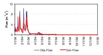
**Fig. 3.** Measured and simulated streamflow at gauge 2. Validation (1994).
