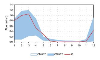
**Fig. 5.** Natural streamflow (25<sup>th</sup> and 75<sup>th</sup> percentiles) and actual monthly median streamflow (Q) at River Section 1.
