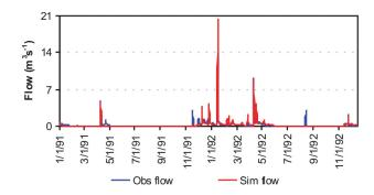
**Fig. 2.** Measured and simulated streamflow at gauge 1. Calibration (1991–1992).
