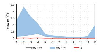
**Fig. 6.** Natural streamflow (25<sup>th</sup> and 75<sup>th</sup> percentiles) and actual monthly median streamflow (Q) at River Section 2.
