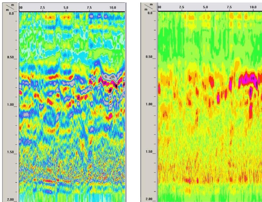
Fig. 2 Ideal case: detection of freshwater limestone's presence based on the electromagnetic wave magnitude
