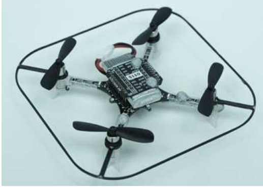
Fig. 2. Crazyflie 2.0 with passive markers and a protective shroud
