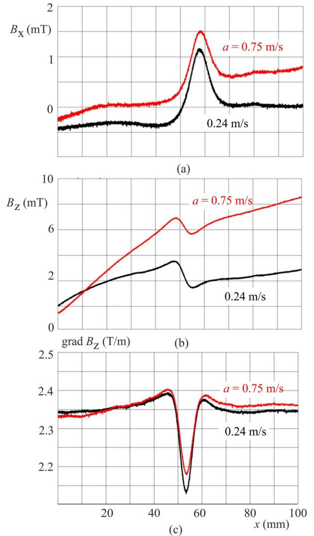
**Fig. 5.** Comparison of waveforms for (a) – the tangential component, (b) – the normal component, and (c) – the gradient obtained for different values of acceleration of the MFL tool. Portions of the signals obtained in the vicinity of the 2 mm deep flaw are presented
