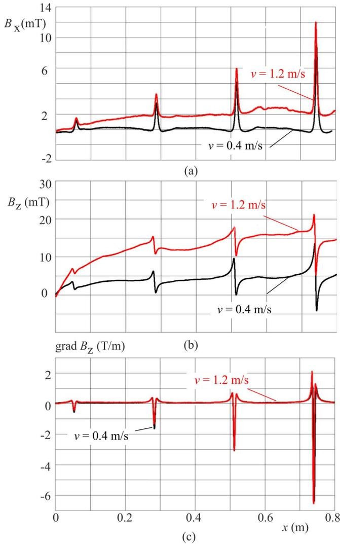
**Fig. 4.** Comparison of waveforms for (a) – the tangential component, (b) – the normal component, and (c) – the gradient obtained for different values of average velocity of the MFL tool
