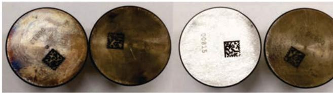
Fig. 2. Samples of DMX code marked with laser on metal surface
