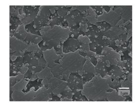
Fig. 1. Microstructure of the nanocomposite containing  $10\,\mathrm{vol\%\,SiC}$
