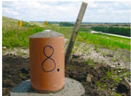
Figure 5. Settlement measuring point.
