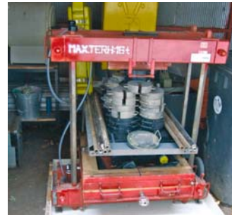
(b) The small loads (large loads were added hydraulically).
