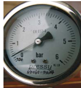
(f) the lateral stress measuring gauges
