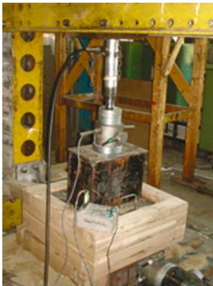
Figure 8. Direct shear test for waste (after [7])
