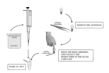
Fig. 1. The scheme of the modified technique of collecting hemolymph flowing out after detachment of the antennae with use of a glass capillary.
