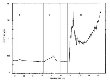
Fig. 2. Differential scanning calorimetry (DSC) heating thermogram of polyfloral honey in the crystallised state in the range of temperatures from -65°C to 220°C; heating rate 10°C/min.
