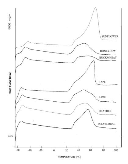
Fig. 3. Differential scanning calorimetry (DSC) heating thermograms of various honeys - 1<sup>st</sup> heating cycle in the range of temperatures from -65°C to 100°C; heating rate 10°C/min.
