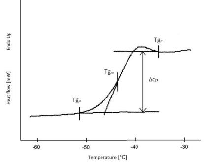
Fig. 1. Determination of glass transition temperatures by differential scanning calorimetry (DSC): onset temperature ( $Tg_o$ ), midpoint temperature ( $T_m$ ), and endpoint temperature ( $Tg_e$ ), and change in specific heat capacity ( $\Delta$ Cp).
