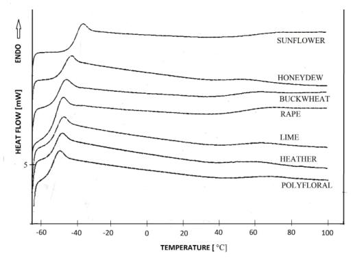
Fig. 4. Differential scanning calorimetry (DSC) heating thermograms of various honeys - 2<sup>nd</sup> heating cycle after decrystallisation in the range of temperatures from -65°C to 100°C; heating rate 10°C/min.
