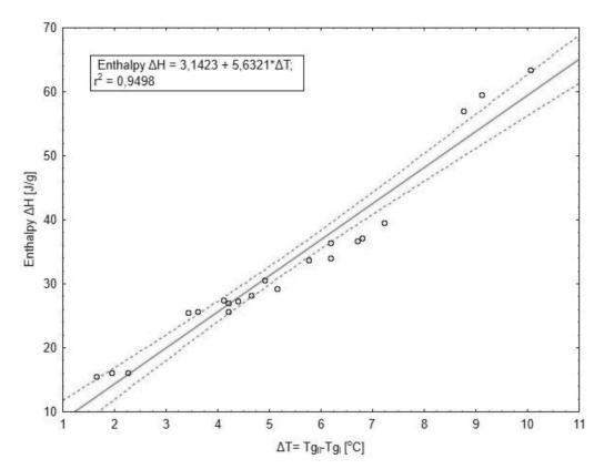
Fig. 5. Relationship between enthalpy ( $\Delta$ H) and difference in glass transition temperatures between 1<sup>st</sup> and 2<sup>nd</sup> cycle of heating ( $\Delta$ T = TgII - TgI). TgI and TgII - glass transition temperatures I and II.
