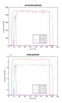
Fig. 5. Difference of number of packets by the firewall a) received and b) transmitted to the network.
