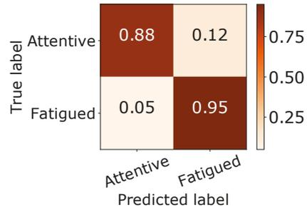
**Figure 16.** Normalized CM of the SVM fatigue model
