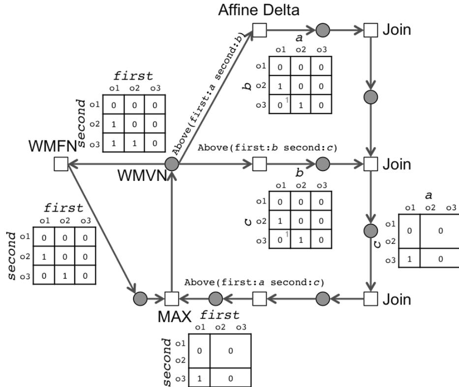
Figure 63: Abstracted factor graph and message passing for the transitive rule in Figure 15, given an initial working memory of *Above*(*first*:*o1* *second*:*o2*) and *Above*(*first*:*o2* *second*:*o3*).
