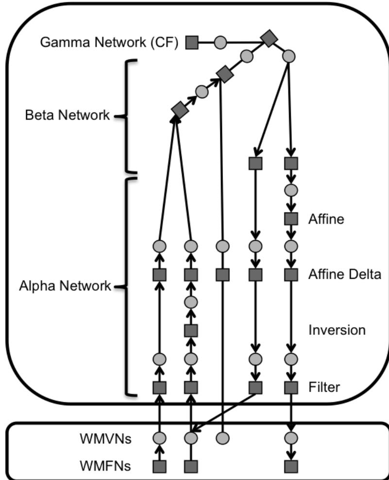
Figure 60: Graph for a conditional with two conditions (left two alpha networks, with arrows pointing away from WM), one contact (middle alpha network, with undirected links), two actions (right two alpha networks, with arrows pointing towards WM), and a function (CF). Four distinct predicates are involved, with the second one supporting both a condition and an action.
