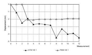
Figure 3. Development of the vertical displacements of the point VB1 measured on the geodetic marks on the embankment and in the FEM model
