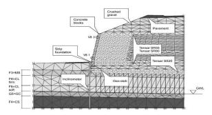
Figure 1. Model for the FEM modelling with the inclinometer and the geodetic marks
