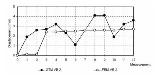
Figure 4. Development of the vertical displacements of the point VB2 measured on the geodetic marks on the embankment and in the FEM model
