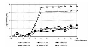
Figure 2. Development of the transversal displacements in the inclinometer and in the FEM model in the depth of 2, 4 and 7 m under the terrain
