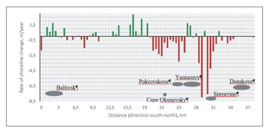
Fig. 3. Shore dynamics of the western shore of the Sambia Peninsula in 2007–2017: mean annual rates of retreat (red) and advance (green), values within confidence limits are yellow. The shore opposite Donskoe is under permanent erosion, but it is excluded from the analysis for lack of data
