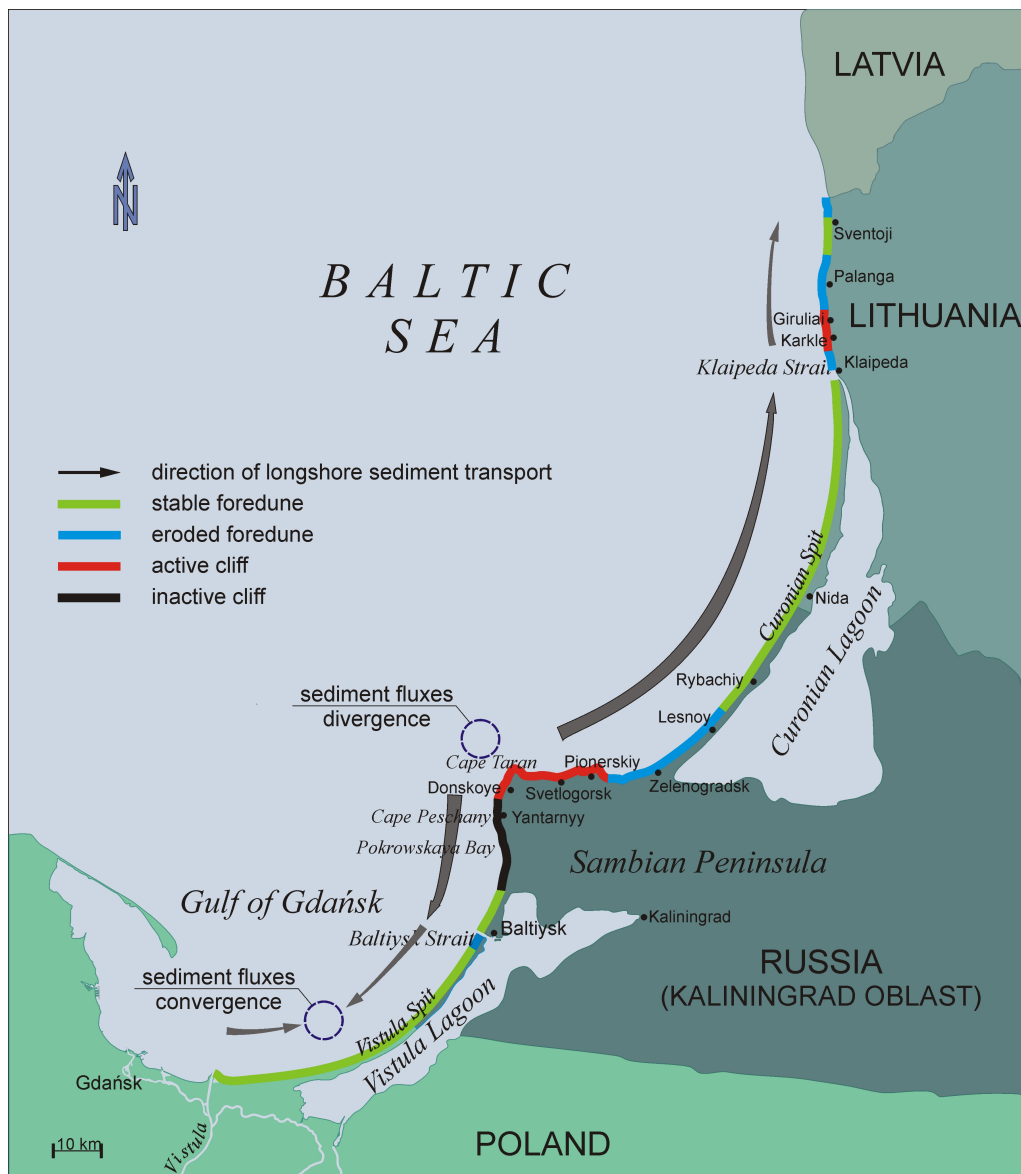
Fig. 15. Longshore sediment transport directions and morphological types of shores in the study area
