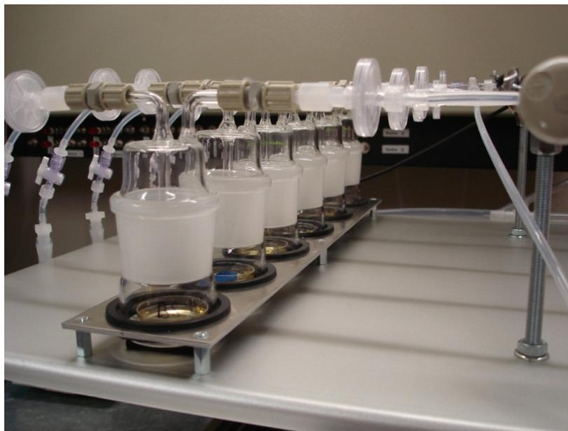
**Figure 1. (A) Cultivation station with 12 custom-built gas vessels in which the organisms are grown under controlled gaseous environments. The E-Nose is connected on the left for measurement of the cultures. (B) Gas vessels with the culture of *Bacillus subtilis* in liquid tryptic soy broth media.**
