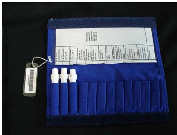
**Figure 4.** Surface Pipette Kit used for swabbing the surfaces of the three locations of measurements. Cotton swabs (Q-tip style) from left to right: Q1: working table, Q2: sleeping cabin, and Q3: toilet lid.
