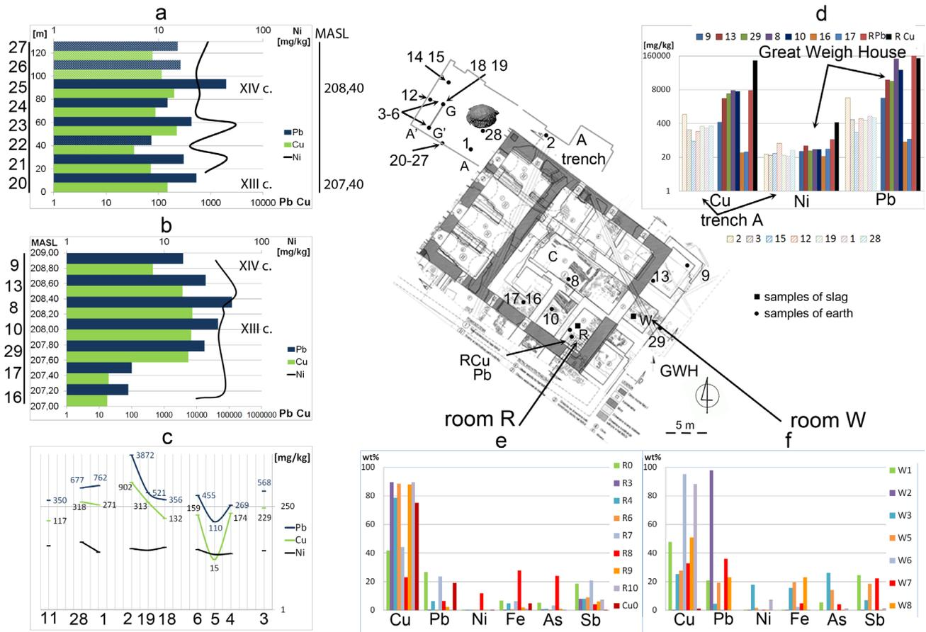
**Fig. 5.** The graphs show elemental content (%wt.) of various samples (as labelled) taken from locations indicated on the plan in the centre (Szejbald-Dereń and Garbacz-Klempka, 2010).
