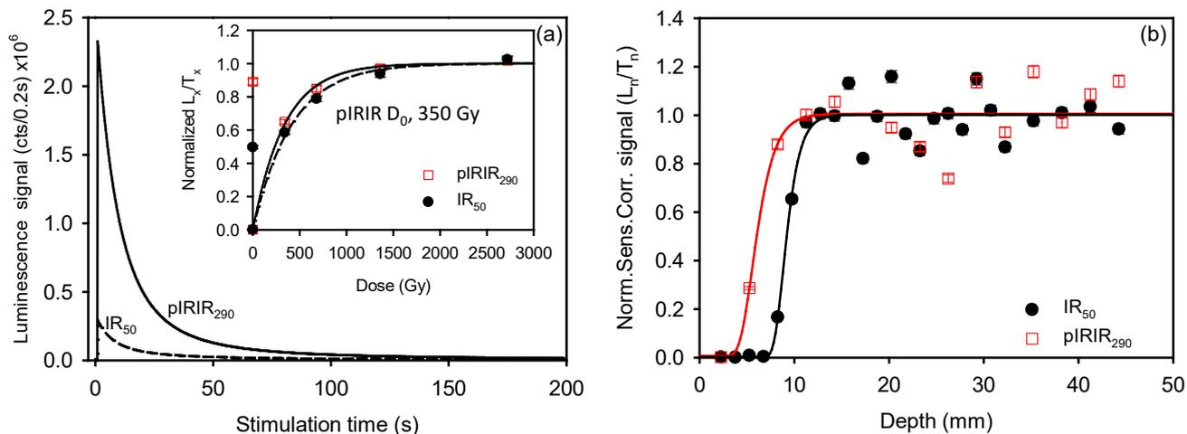
**Fig. 2.** (a) Typical decay curves and (inset) dose response curves of IR<sub>50</sub> (dashed line) and pIRIR<sub>290</sub> (solid line) signals. (b) The variation of the IR<sub>50</sub> and pIRIR<sub>290</sub> "residual signals" with depth into the rock surface.
