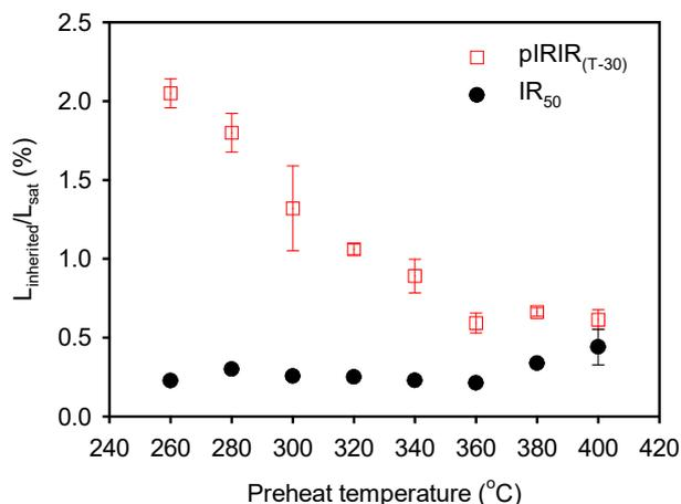
**Fig. 3.** The ratio of the "residual signal" (steps 1-5, 1-6, Table 1B) to the initial signal (steps 1-3, 1-4) at different preheat and stimulation temperatures. Three slices were measured at each temperature. The error bars represent one standard error.
