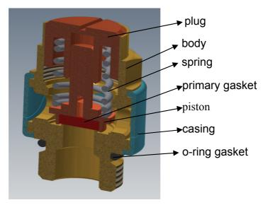
Figure 3. The safety valve, which is the subject of the new project in the R&D department in the manufacturing company
