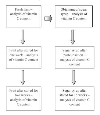
Figure 2. Schematic diagram of the experiment
