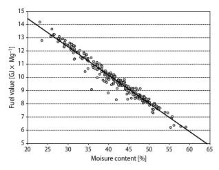
**Figure 2.** Relationship between the fuel value of forest wood chips and their humidity
