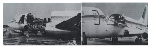
Fig. 7. Boeing 737 from Aloha Airlines after the accident [33]
