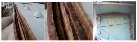
Fig. 2. Crevice corrosion on steel elements [21]
