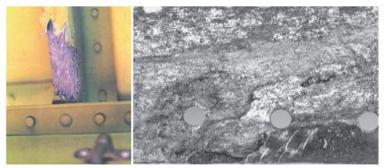
Fig. 4. Exfoliation corrosion [22] [23]
