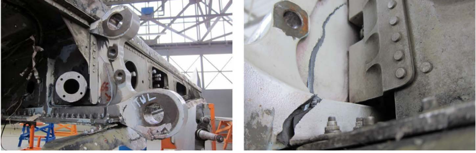
Fig. 1. Critical damage in the Full Scale Fatigue Test
