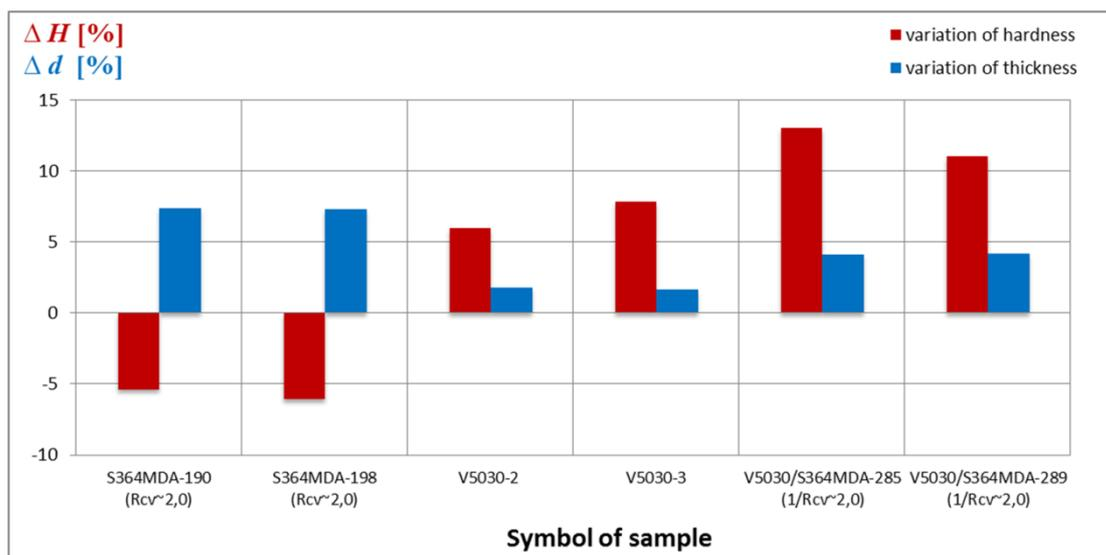
Fig. 6. Determined values of thickness and hardness change for S364MDA auxetic samples ( $R_{CV} \sim 2.0$ ), V5030 viscoelastic foam samples and 2-layered structures composed of S364MDA and V5030 foams
