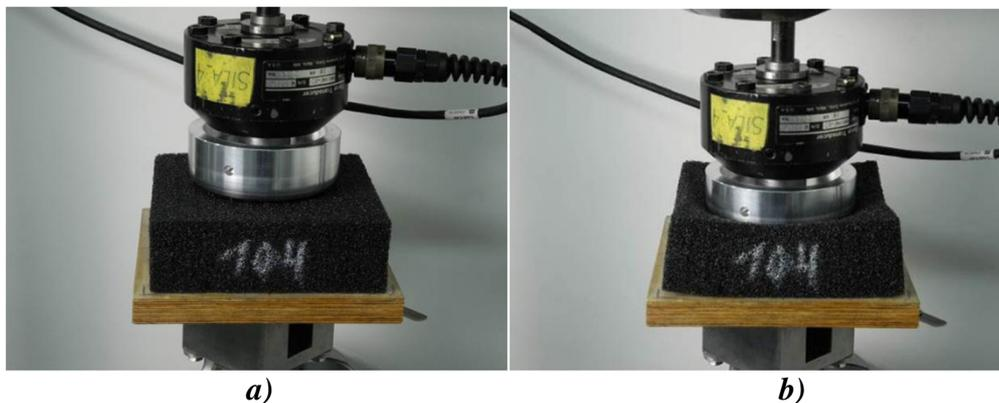
**Fig. 2. Indenter and S28280 auxetic foam sample:
