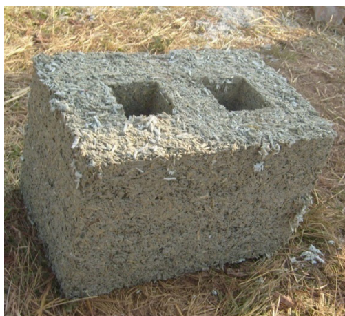
Figure 6. A prefabricated element in the form of a block of lime-hemp composite
