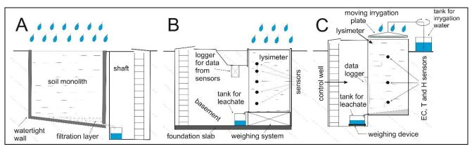
Fig. 1. Examples of lysimeter construction
