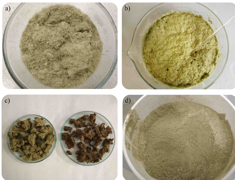
Fig. 2. Decalcification procedure for removal of calcium carbonate incrustations from Cladophora glomerata ; a) dry algal biomass before the acid wash, b) during acetic acid wash, c) comparison between material treated with acetic (left) and citric acid (right), after drying, with evident degradation of plant pigments in the latter case, d) pulverized, decalcified biomass after acetic acid wash and drying, already ground together with disodium EDTA
